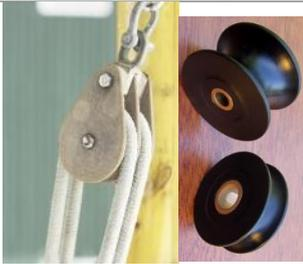
A sheave is one of the components of a pulley. It is, very often, a wheel with a groove along its surface through where a belt, a rope, or a cable passes through.
