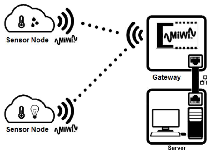
Figure 3 – The NSensor WSN configuration
