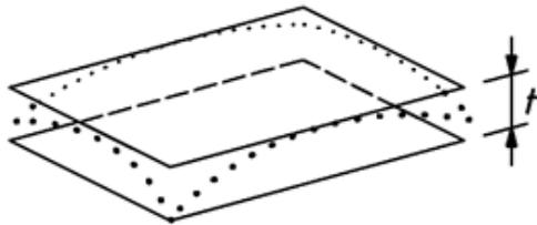
*Definition of the flatness tolerance zone of a flat surface*
